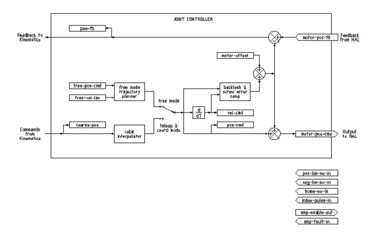
Figure 3.1 - Joint Controller Block Diagram
