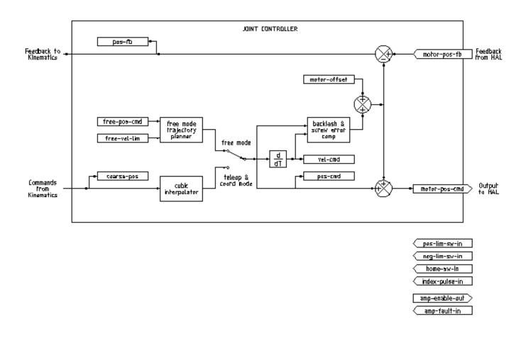
Figura 3.1: Joint Controller Block Diagram
