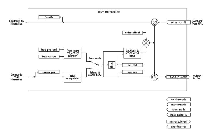
Figura 3.1: Joint Controller Block Diagram
