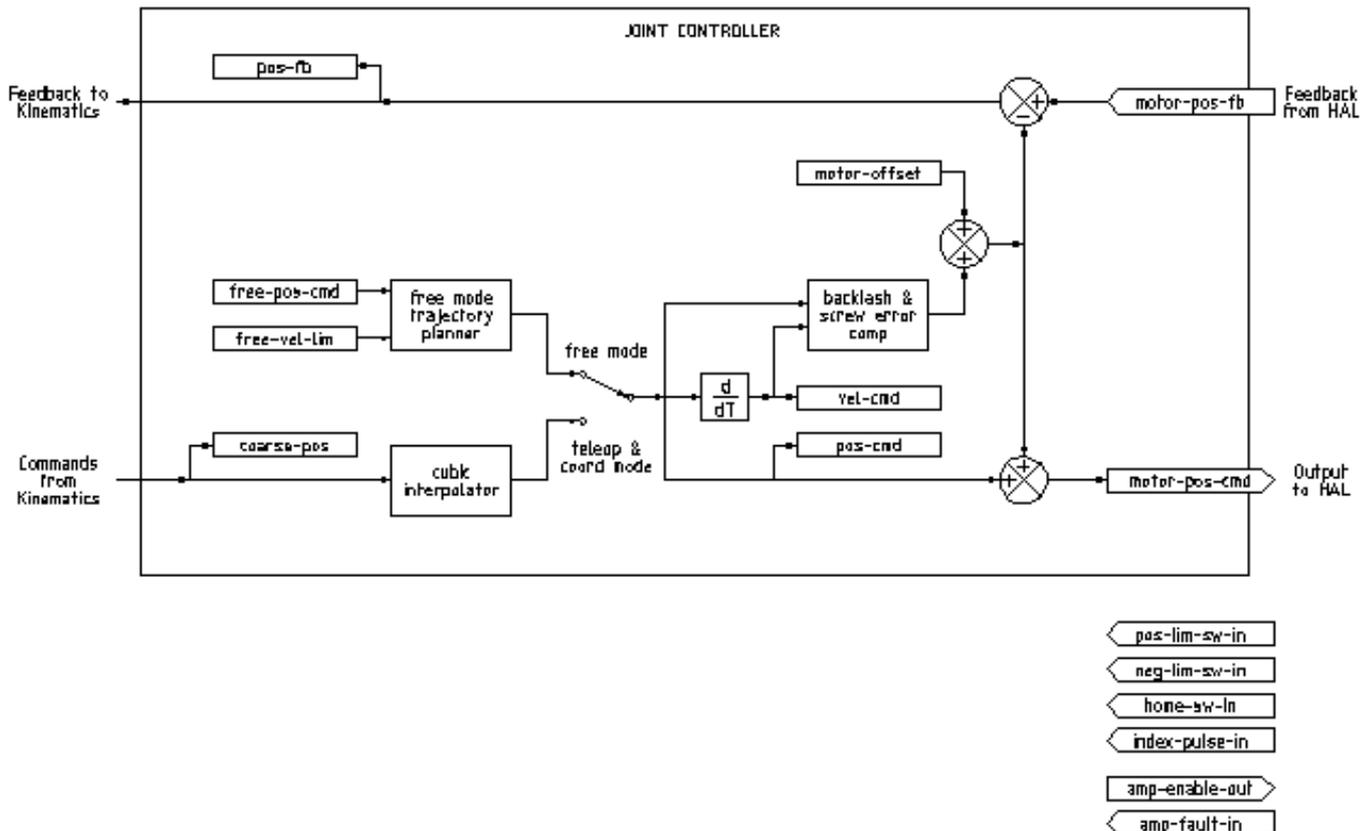
Figure 3.1: Joint Controller Block Diagram
