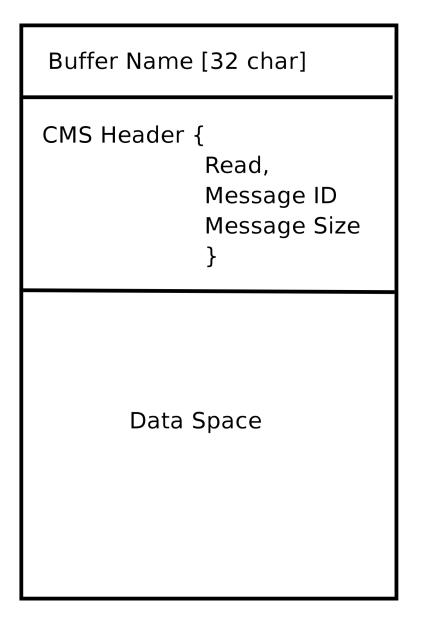
**CMS buffer** The CMS base class is primarily responsible for creating the communications pathways and interfacing to the operating system.
