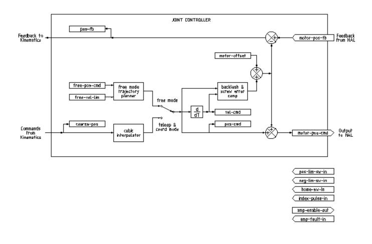
Figura 3.1: Joint Controller Block Diagram
