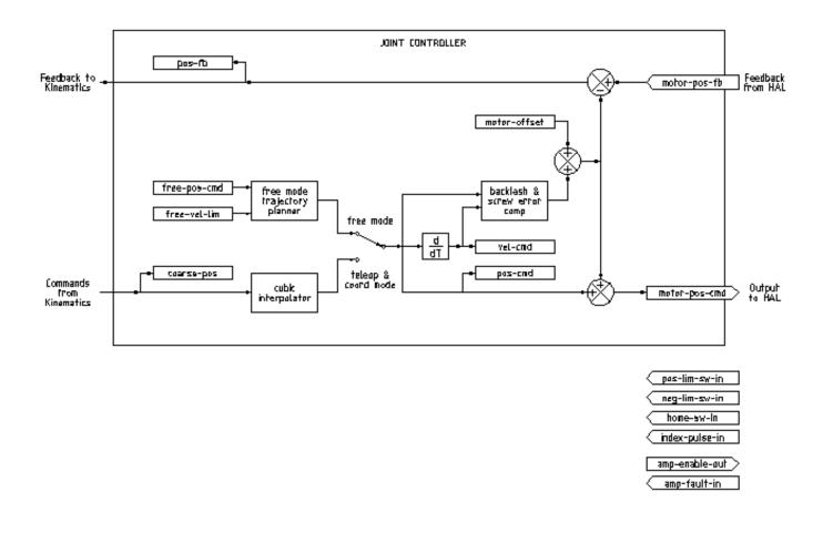
Figure 3.1 - Joint Controller Block Diagram
