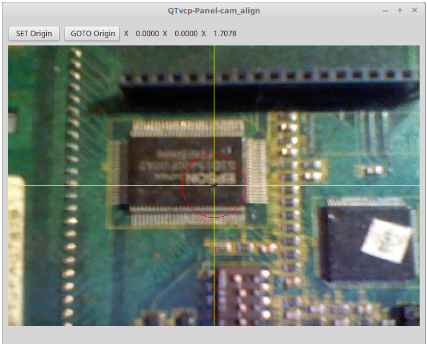
Figure 12.74: QtVCP cam_align Panel - Camera Based Alignment Panel
