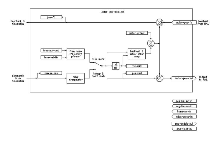
Figure 3.1 - Joint Controller Block Diagram
