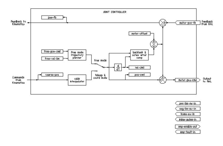
Figure 3.1: Joint Controller Block Diagram
