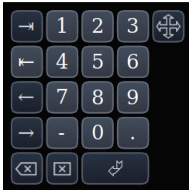
Figure 10.47: Number keypad - used for the CONVERSATIONAL Tab and the PARAMETERS Tab
