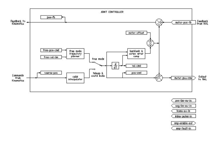
Figur 3.1: Joint Controller Block Diagram
