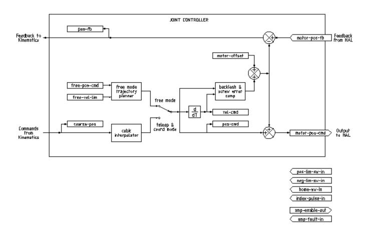
Figure 3.1 - Joint Controller Block Diagram
