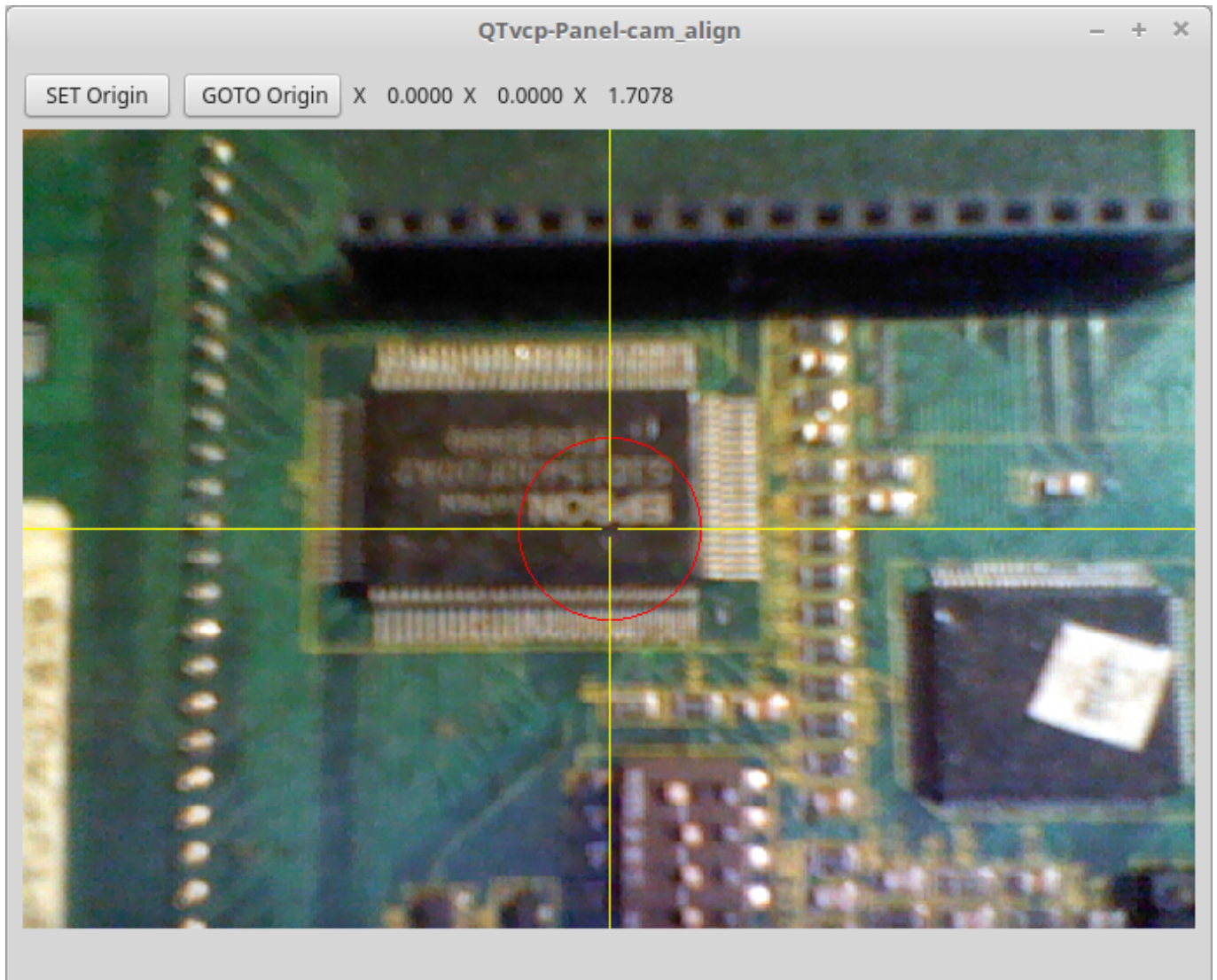
Figure 12.63: cam_align - Camera Alignment VCP
