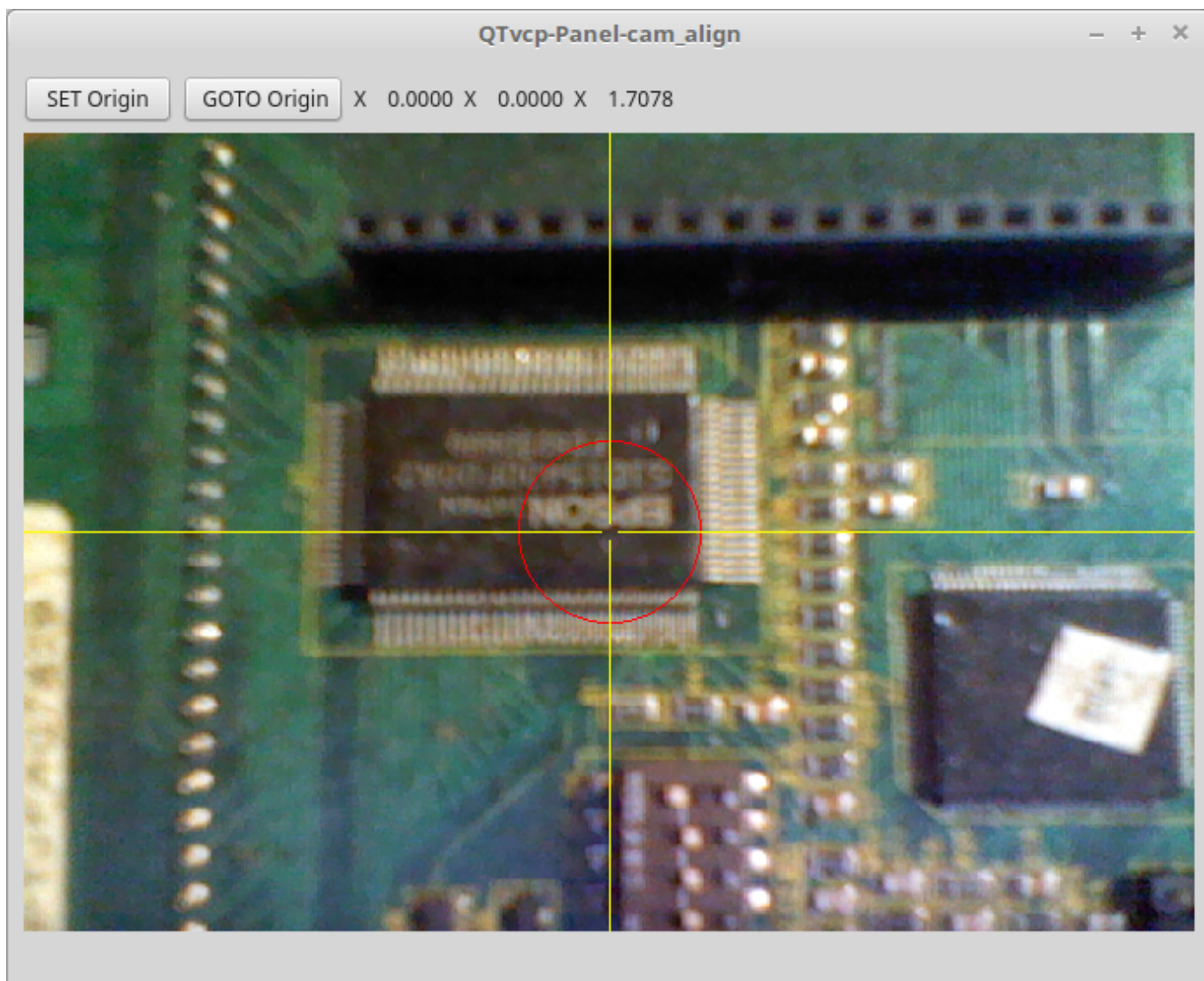
Figure 12.63: cam_align - Camera Alignment VCP
