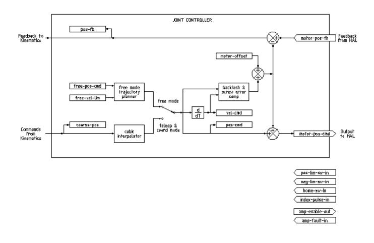
Figure 3.1 - Joint Controller Block Diagram
