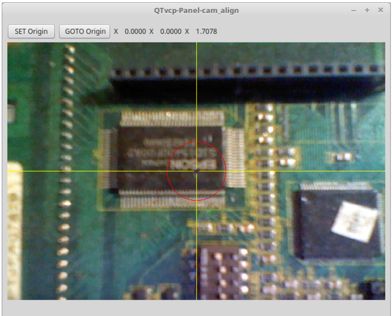
Figure 12.74: QtVCP cam_align Panel - Camera Based Alignment Panel
