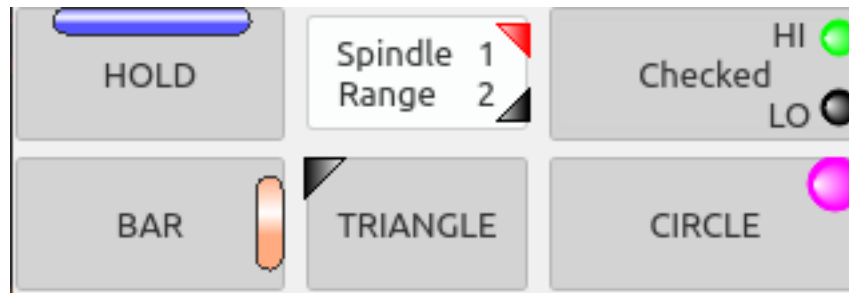
Figure 12.109: QtVCP QPushButton: IndicatedPushButton Button, LED Indicator Option
