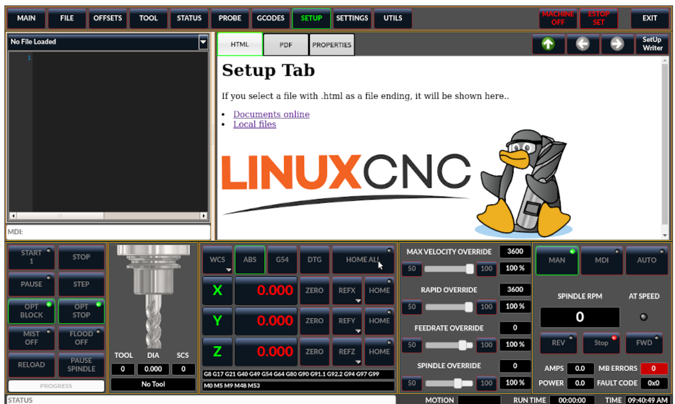
Figure 10.34: QtDragon - Setup Tab Sample
