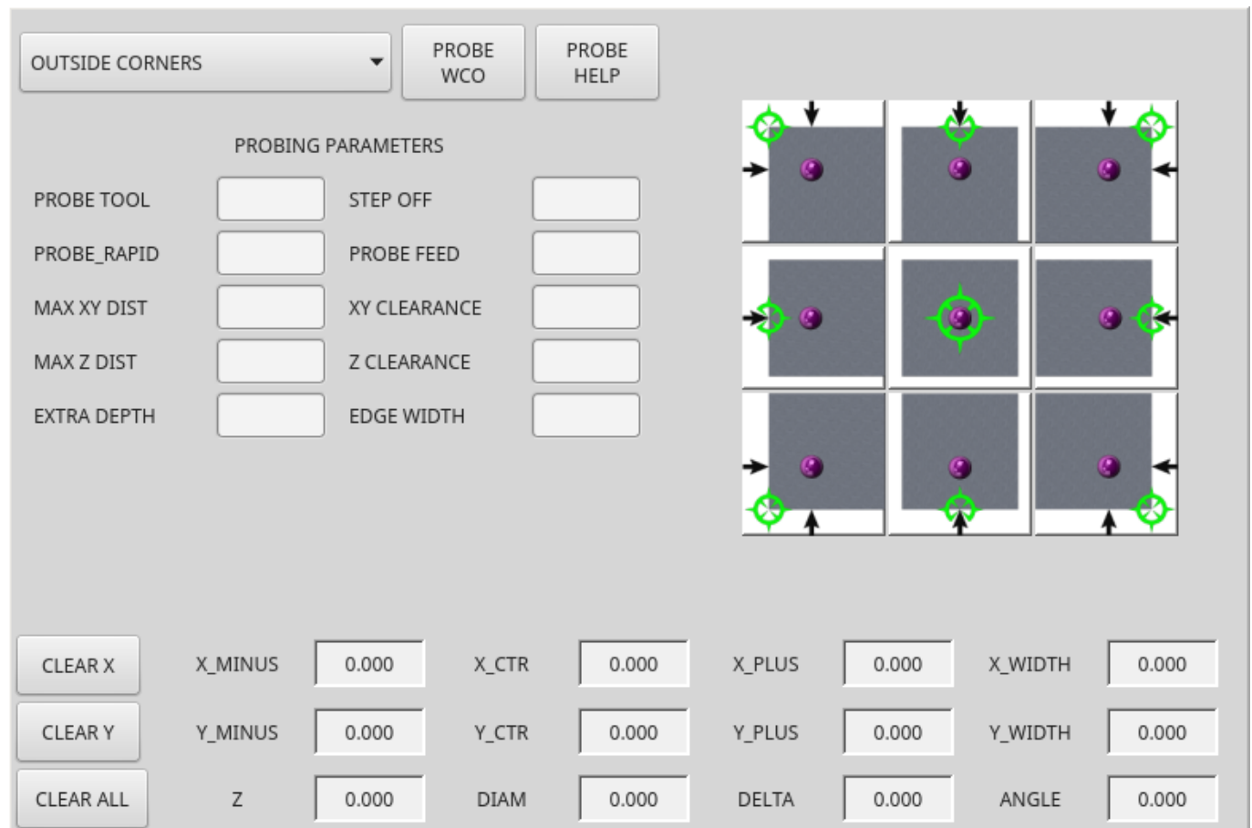
Figure 12.88: QtVCP BasicProbe: Simple Mill Probing Widget
