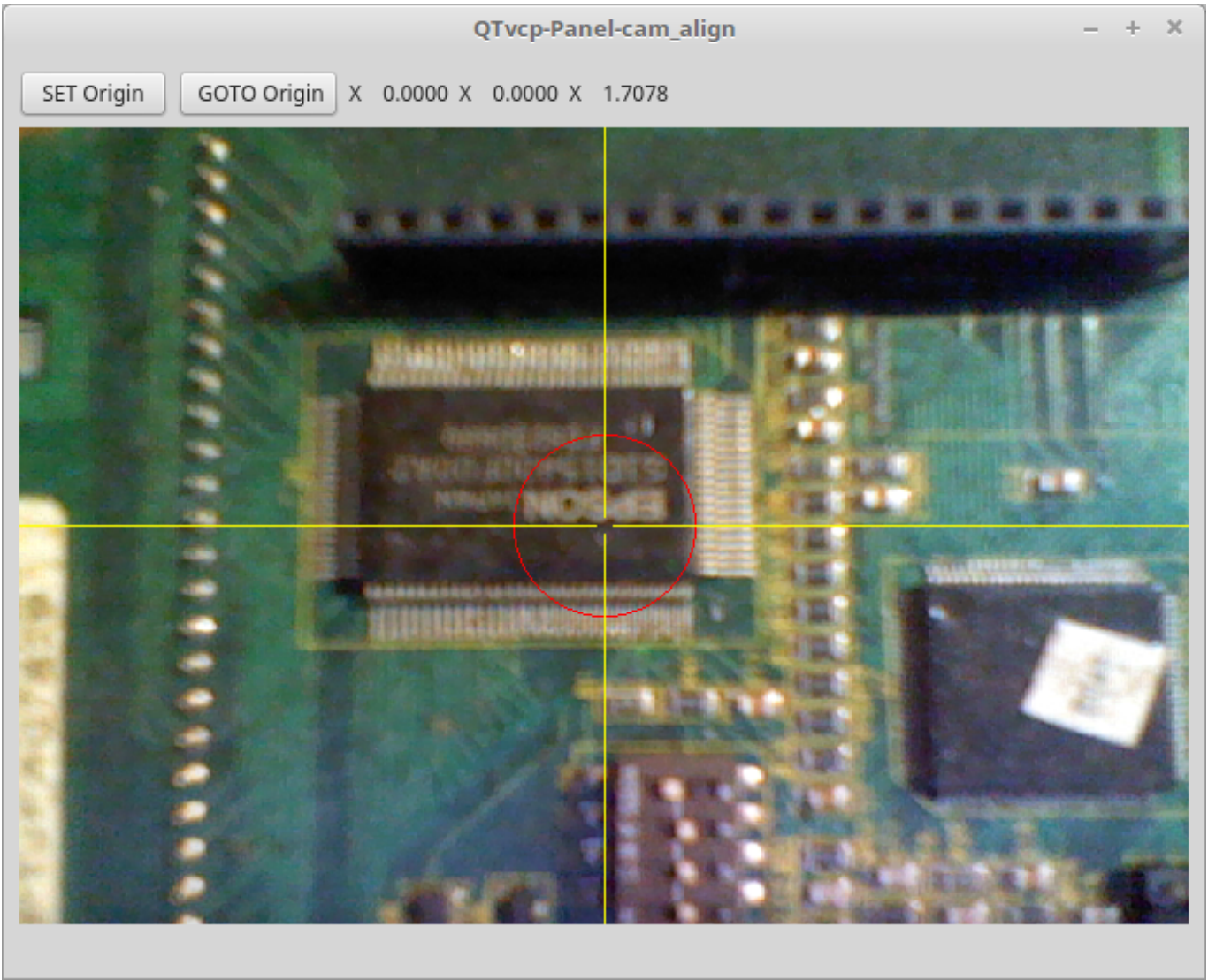
Figure 12.60: cam_align - Camera Alignment VCP
