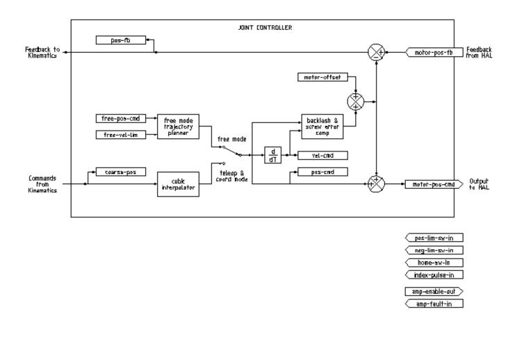
Figura 3.1: Joint Controller Block Diagram
