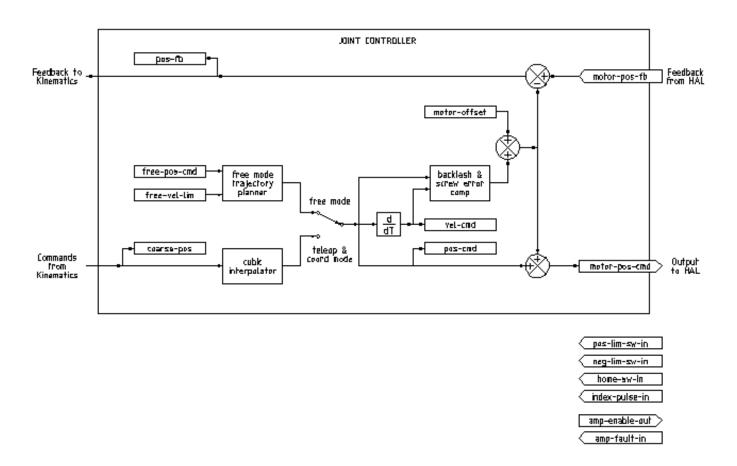
Figure 3.1: Joint Controller Block Diagram
