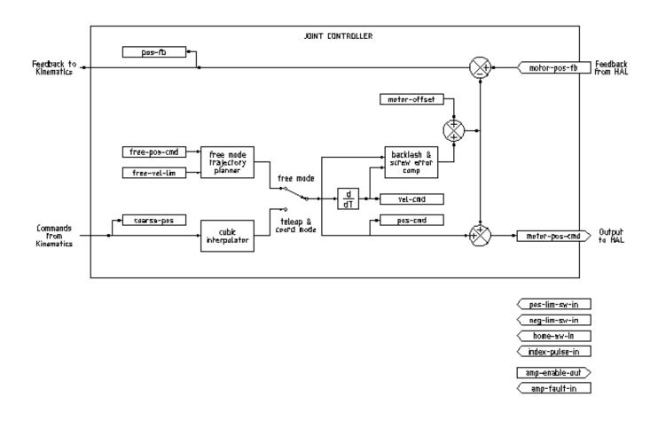
Figure 3.1 - Joint Controller Block Diagram
