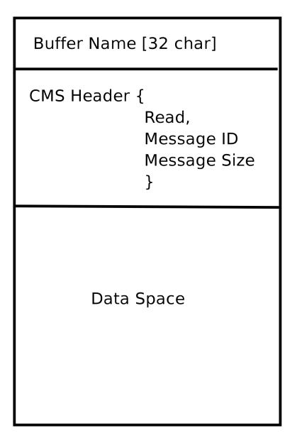
$\mbox{CMS}$  buffer The CMS base class is primarily responsible for creating the communications pathways and interfacing to the operating system.
