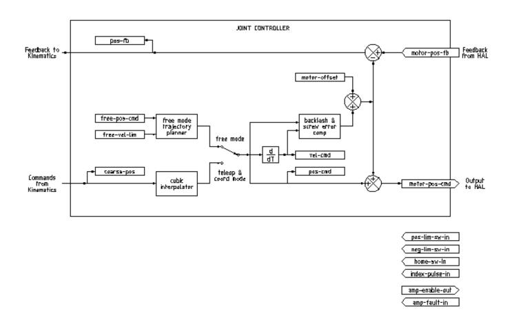
Figur 3.1: Joint Controller Block Diagram
