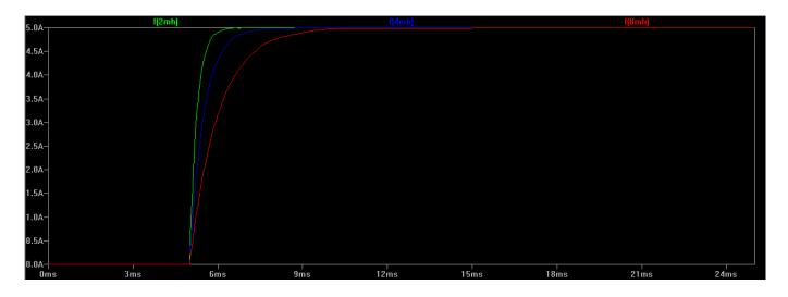
If the rate at which step changes are applied to the coils is significantly shorter than the rise time, it's easy to see that the winding has less time to attain full magnetic attraction on the rotor, and thus maximum torque is curtailed. In the below example the 2 mH coil can achieve the full 5 A limit before the step voltage is removed, but the 4 mH and 8 mH coils cannot:
