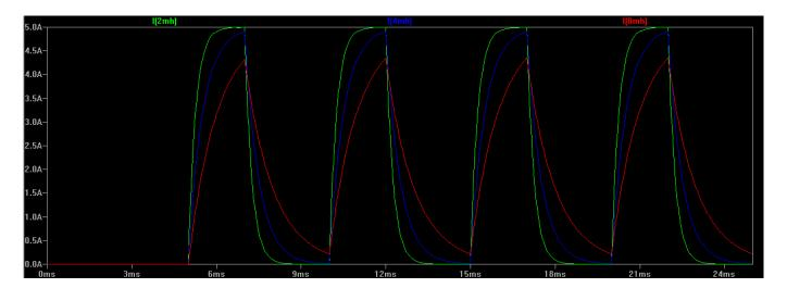
The accepted way of improving motor speed while maintaining torque is to increase the speed at which the magnetic field of the motor coils can expand and collapse. The easiest way to accomplish this is to increase the supply voltage to force the current in each winding to rise and fall much more rapidly. A guicker magnetising time equates to faster step rates while improving torque at higher speeds, both of which are obviously desirable in a CNC system.
