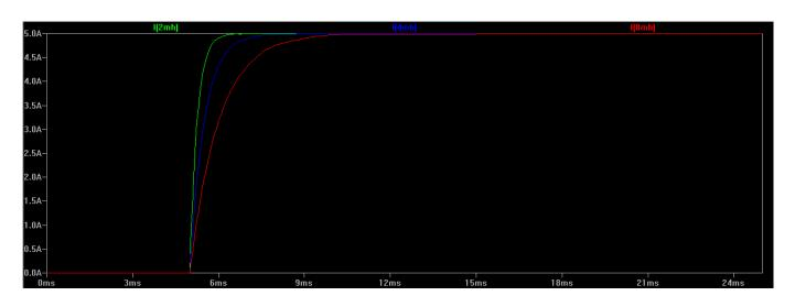
If the rate at which step changes are applied to the coils is significantly shorter than the rise time, it's easy to see that the winding has less time to attain full magnetic attraction on the rotor, and thus maximum torque is curtailed. In the below example the 2 mH coil can achieve the full 5 A limit before the step voltage is removed, but the 4 mH and 8 mH coils cannot:
