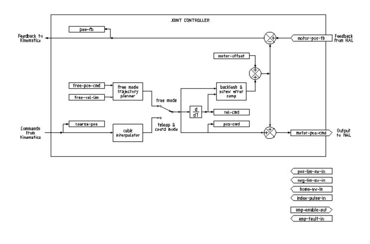
Figure 3.1: Joint Controller Block Diagram
