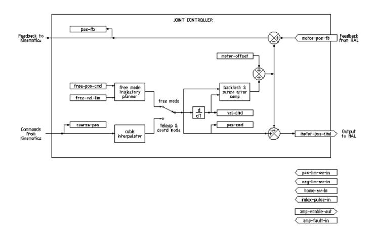
Figure 3.1 - Joint Controller Block Diagram
