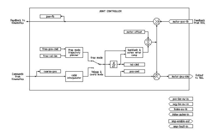
Figure 3.1 - Joint Controller Block Diagram
