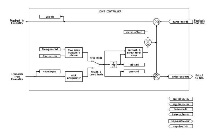
Figure 3.1: Joint Controller Block Diagram
