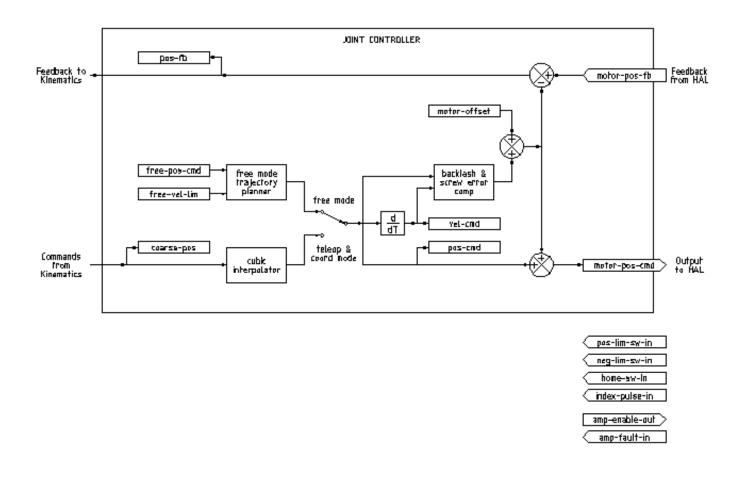
Figure 3.1 - Joint Controller Block Diagram
