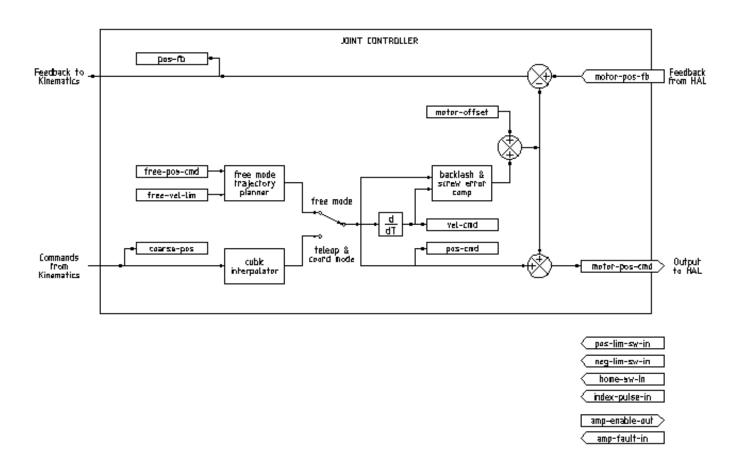
Figura 3.1: Joint Controller Block Diagram
