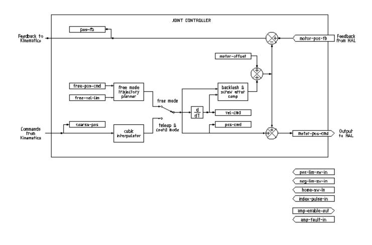
Figure 3.1: Joint Controller Block Diagram
