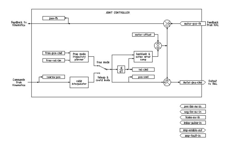
Figure 3.1: Joint Controller Block Diagram
