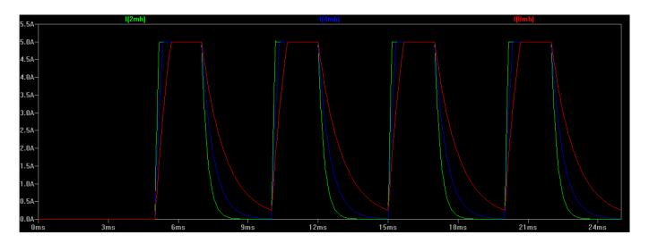
However, careful management of a higher drive voltage is required, as a higher voltage will increase current flowing in each coil with a corresponding increase in temperature of the winding. Excessive temperature rise in the winding will lead to eventual overheating and failure of the motor.
