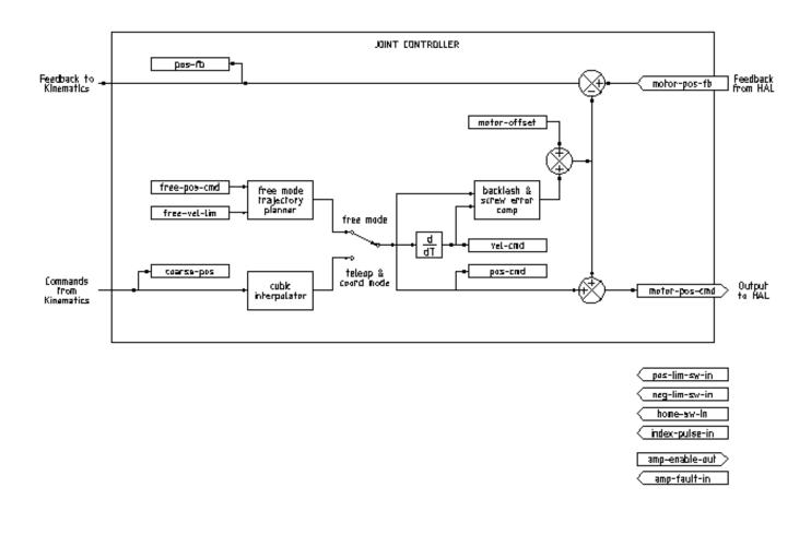
Figure 3.1: Joint Controller Block Diagram
