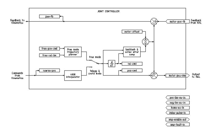
Figure 3.1: Joint Controller Block Diagram
