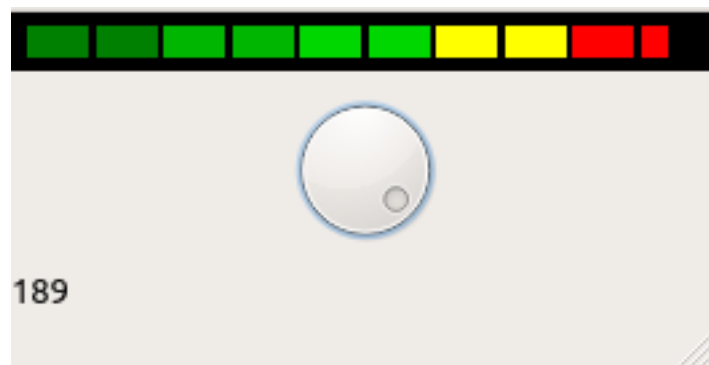
Figure 12.85 - QtVCP HalBar: Panel demonstrating the HAL Bar Level Indicator
