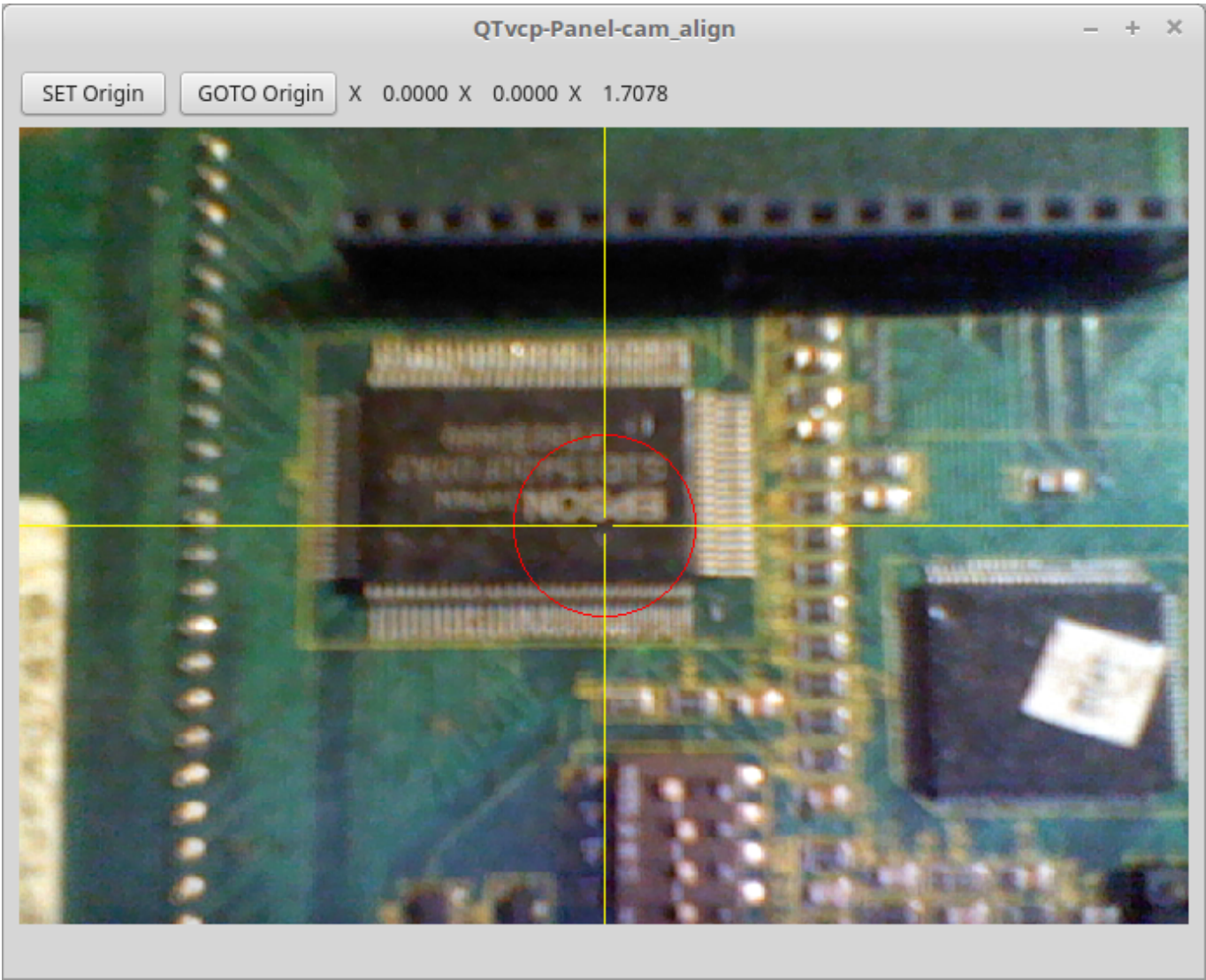
Figur 12.60: cam_align - Camera Alignment VCP
