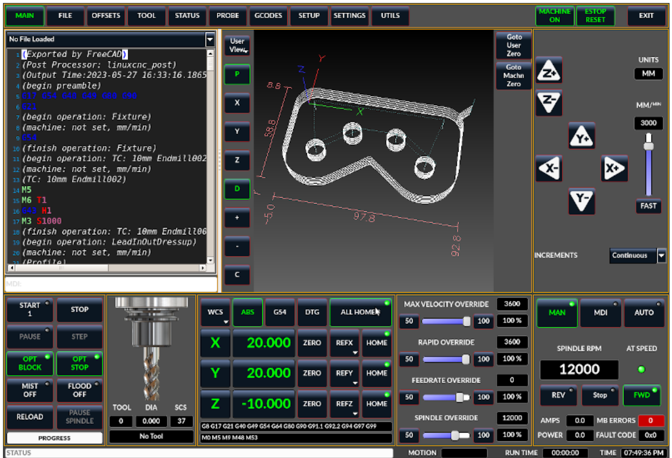
Figure 2.8: QtDragon, a touch screen GUI based on QtVCP
