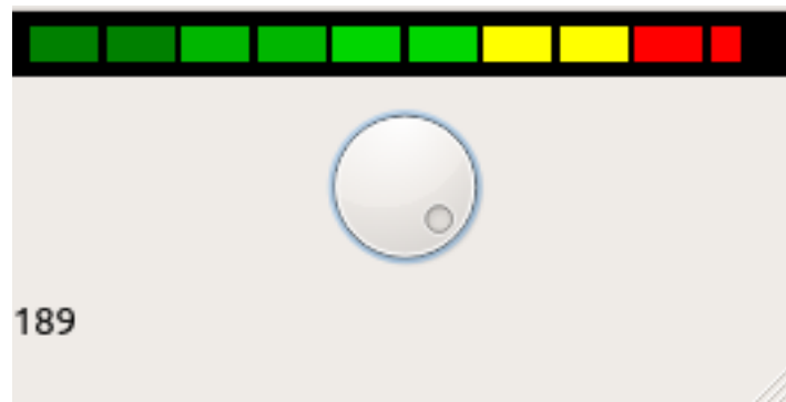
Figur 12.85: QtVCP HalBar: Panel demonstrating the HAL Bar Level Indicator
