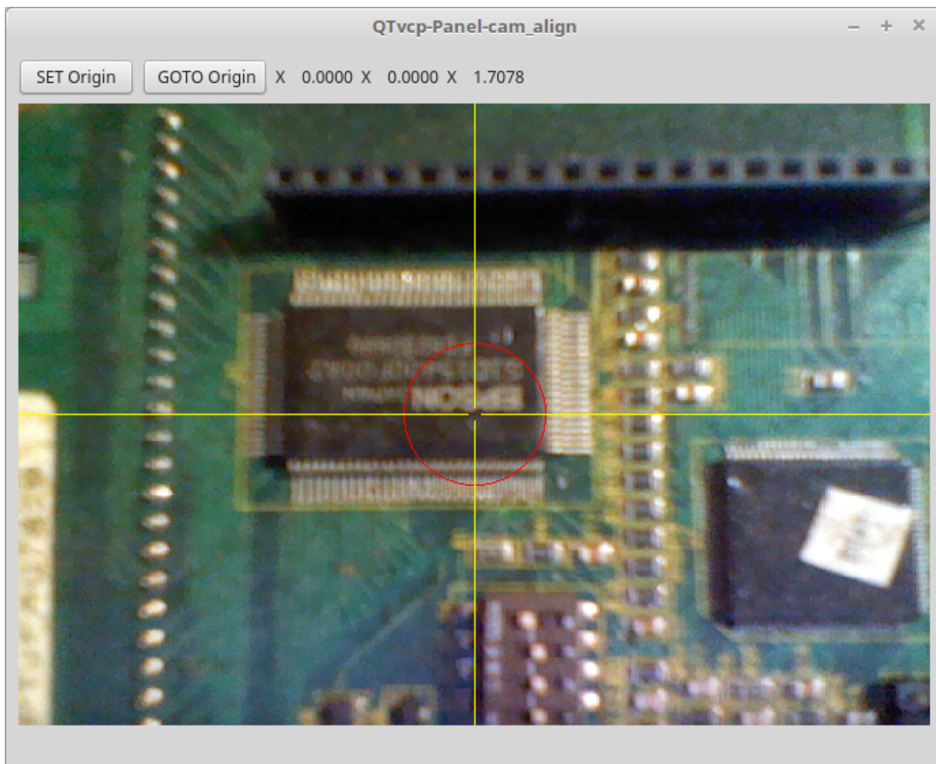
Figur 12.63: cam_align - Camera Alignment VCP
