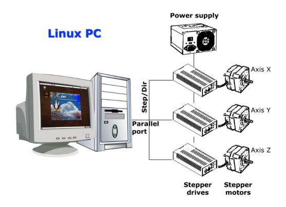
Figure 2.1 - Simple LinuxCNC Controlled Machine
