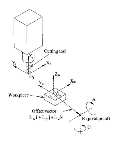
Figure 9.5 - Table tilting/rotary configuration
