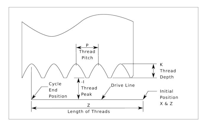
Figure 11.14 - G76 Threading
