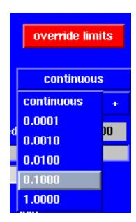
Figure 10.39 - TkLinuxCNC Override Limits & Jogging increments example
