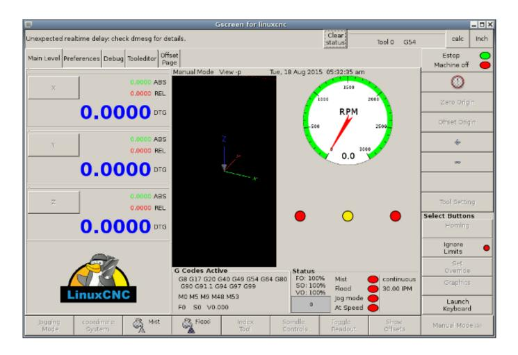
Figure 2.4 - Gscreen, a configurable base touch screen GUI
