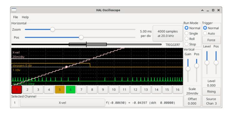
Figure 5.17 - Step Pulses
