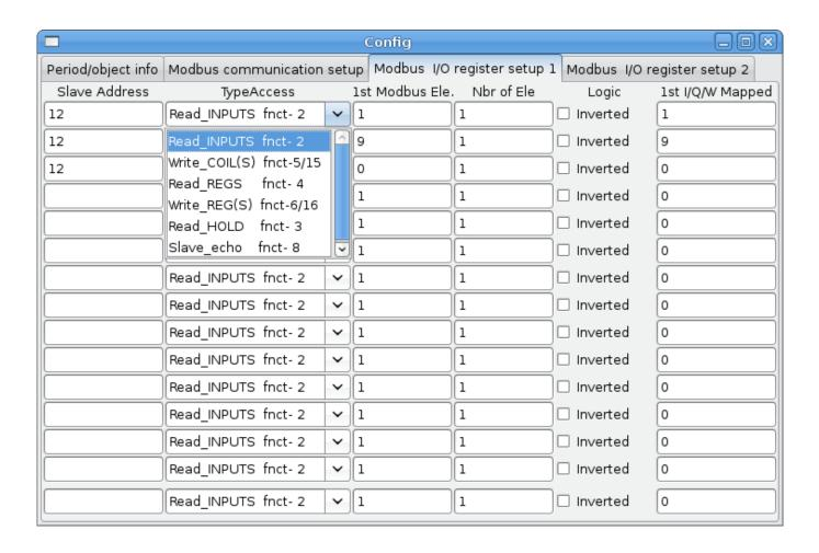
Figure 8.12 - Modbus I/O Config
