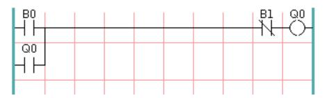
Now we have added *off* or *stop* pushbutton B1. If the user pushes it, contact from the rung to the coil is broken. When coil Q0 loses power, it drops to 0/off/false. When coil Q0 goes off, so does switch Q0, so the *holding contact* is broken, or the circuit is *unsealed*. When the user releases the *stop* pushbutton, contact is restored from the rung to coil Q0, but the rung has gone dead, so the coil doesn't come back on.
