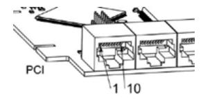
Figure 6.4 - Pin numbering of axis connectors
