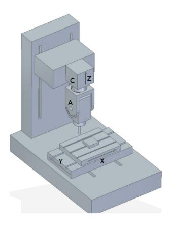
Figure 9.12 - Spindle tilting/rotary configuration
