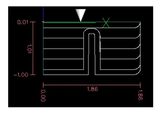
Figure 11.17 - Roughing passes and final pass
