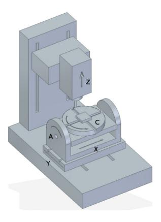
Figure 9.10 - Table tilting/rotating configuration
