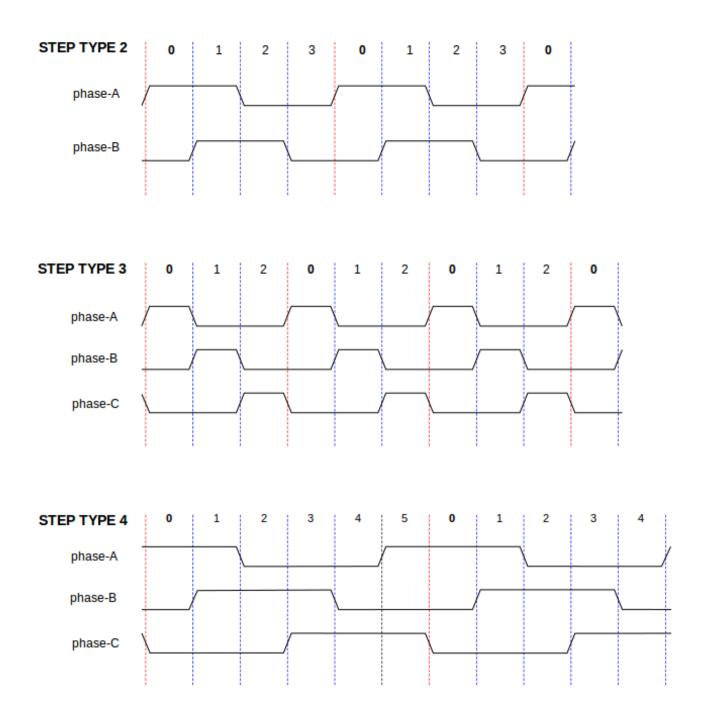
Figure 5.21 - Two-and-Three-Phase Step Types
