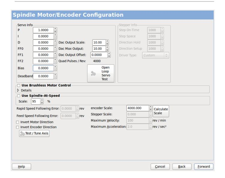
Figure 3.25 - Spindle Motor/Encoder Configuration
