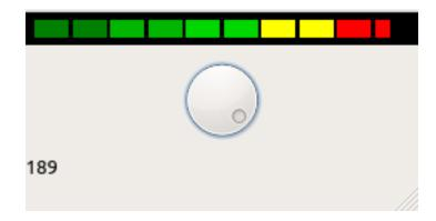
Figure 12.85 - QtVCP HalBar: Panel demonstrating the HAL Bar Level Indicator
