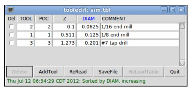
Figure 11.8 - Tool Edit GUI - Column Sorting
