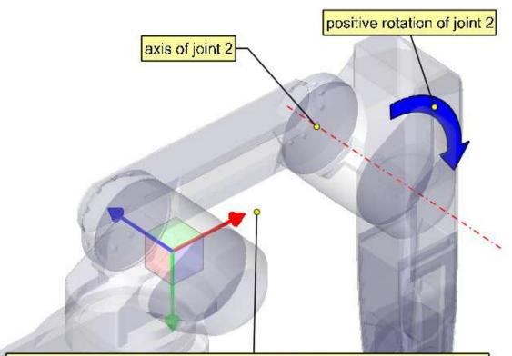
By rotating our joint-1 by 90° we made our X-axis intersect the axis of the next joint and we can continue defining our DH-Parameters.
