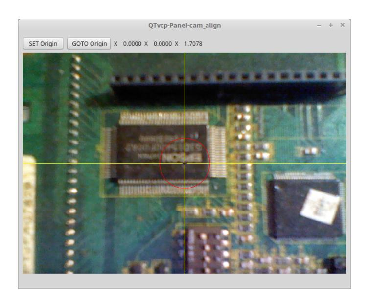
Figure 12.63 - cam\_align - Camera Alignment VCP
