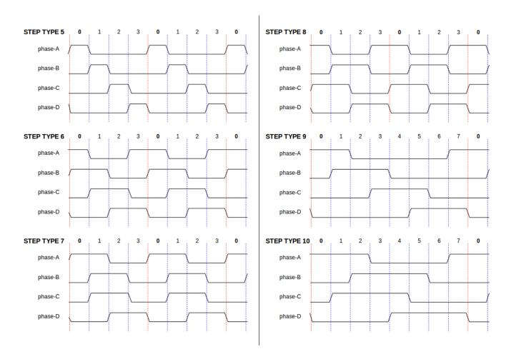
Figure 5.22 - Four-Phase Step Types
