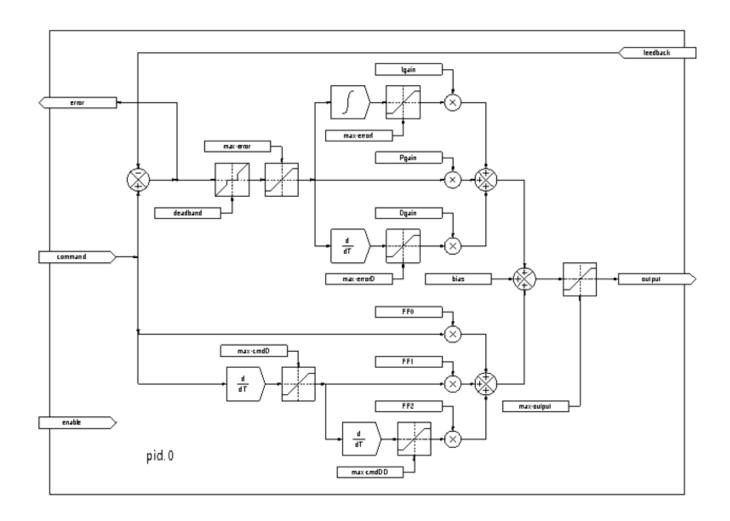
Figure 5.25 - PID Loop Block Diagram
