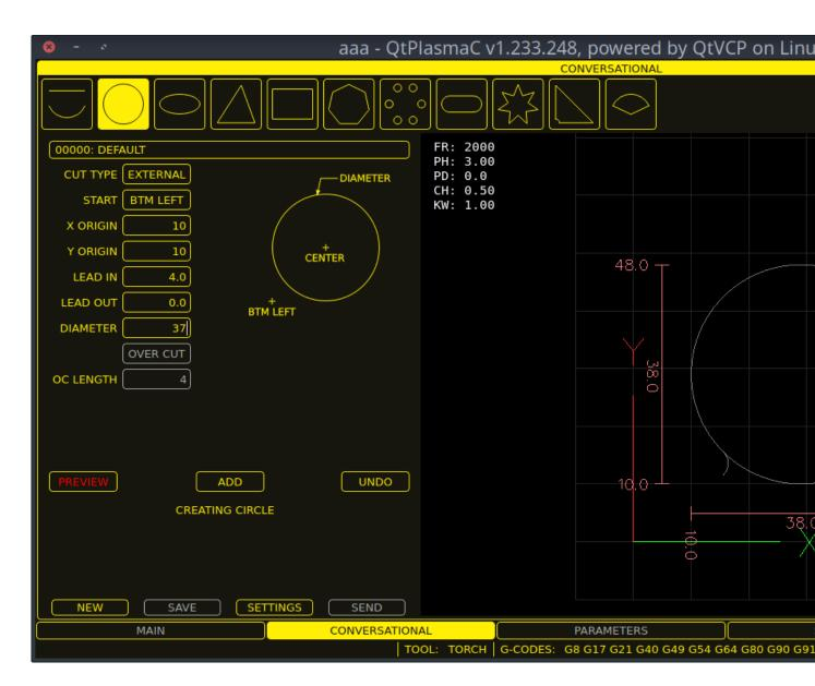
The CONVERSATIONAL Tab enables the user to quickly program various simple shapes for quick cutting without the need for CAM software.
