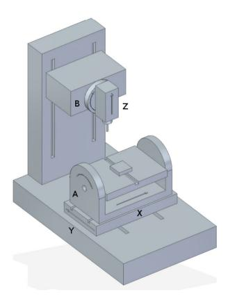
Figure 9.11 - Spindle/table tilting configuration
