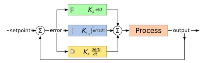
Figure 4.2 - PID Loop
