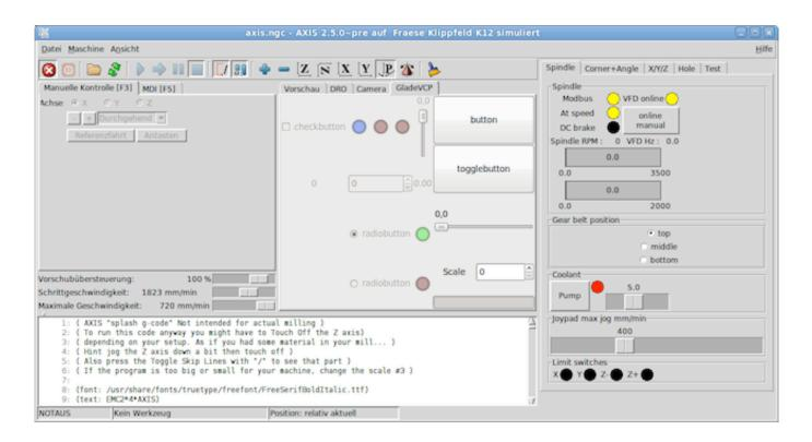
Figure 2.11 - GladeVCP Example Embedded Into AXIS GUI
