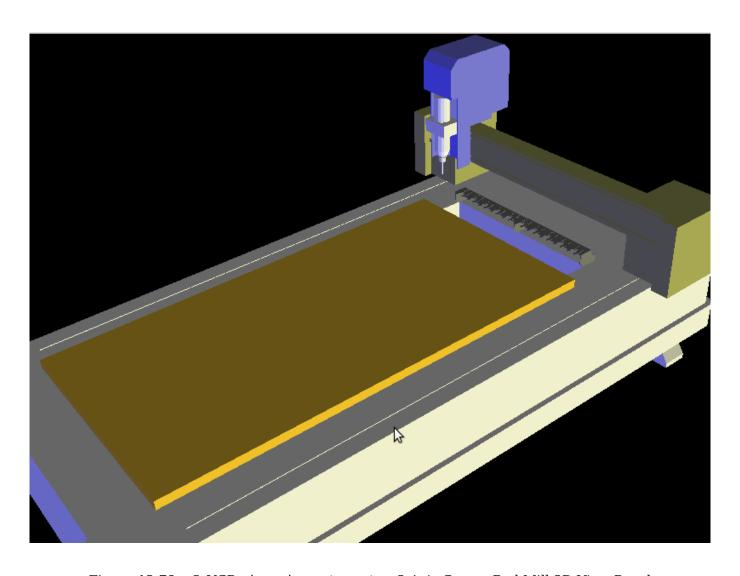
Figure 12.78 - QtVCP vismach\_router\_atc - 3-Axis Gantry Bed Mill 3D View Panel
