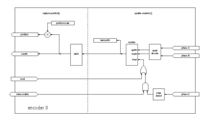
Figure 5.24 - Encoder Counter Block Diagram
