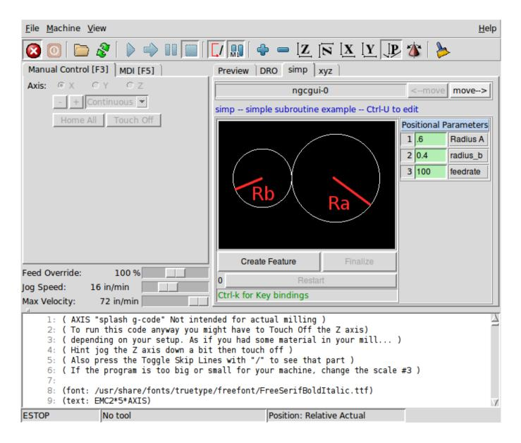
Figure 2.6 - NGCGUI, a graphical interface integrated into AXIS
