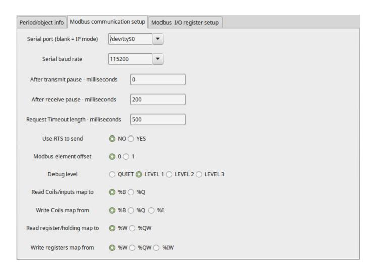
Figure 8.15 - Modbus Communication Setup
