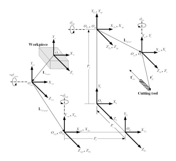
Figure 9.3 - General configuration and coordinate systems
