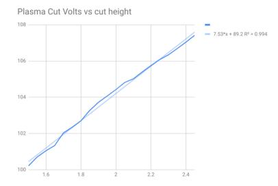
This graph was prepared from a sample of about 16,000 readings at varying cut height and the regression analysis shows 7.53 V/mm with 99.4% confidence. In this particular instance this sample was taken from an Everlast 50 A machine being controlled by LinuxCNC.
