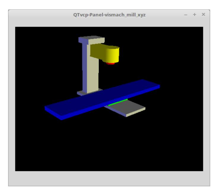
Figure 12.77 - QtVCP vismach\_mill\_xyz - 3-Axis Mill 3D View Panel
