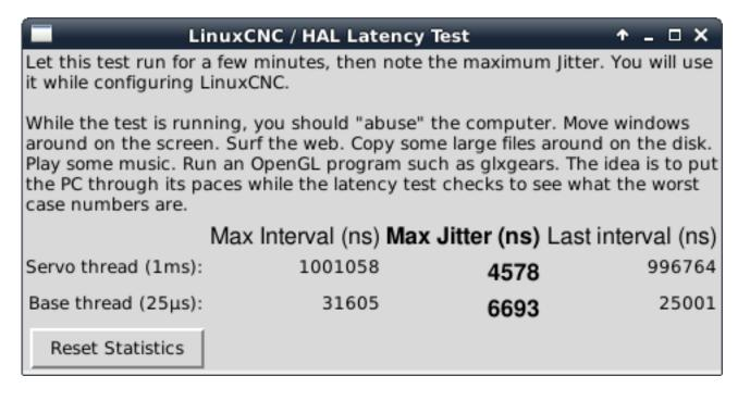
Figure 3.3 - Latency Test
