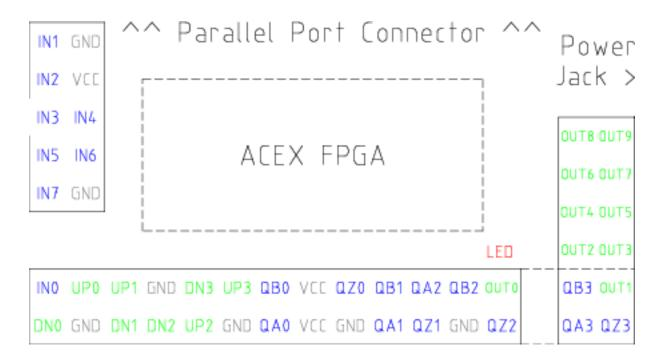
Figure 6.10 - Pluto-Servo Pinout
