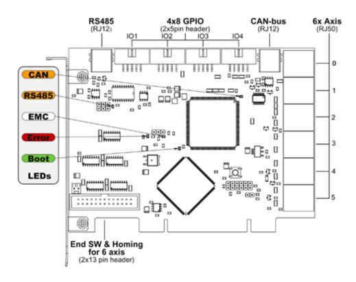
Figure 6.2 - GM6-PCI card connectors and LEDs
