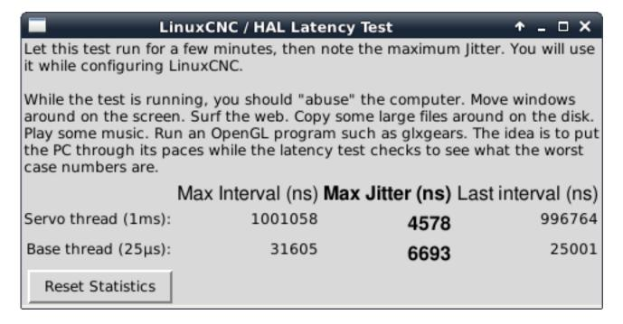
Figure 4.3 - HAL Latency Test
