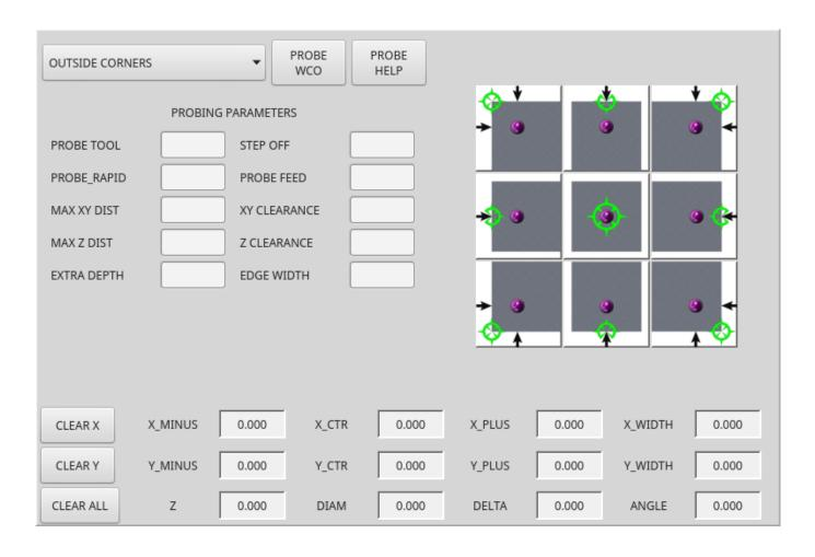
$Figure\ 12.95-QtVCP\ {\tt BasicProbe}; Simple\ Mill\ Probing\ Widget$
