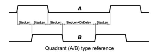
Figure 6.6 - Reference signal timing diagrams
