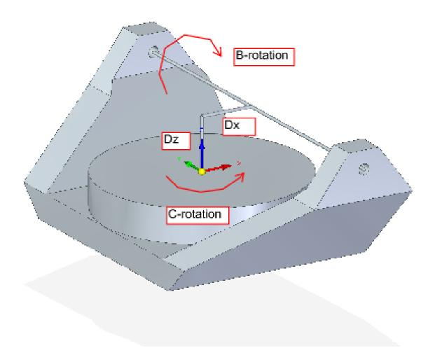
Figure 9.9 - Table tilting/rotary xyzbc-trt configuration, with axis offsets
