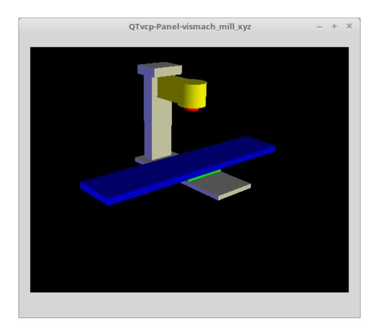
Figure 12.65 - QtVismach - 3-Axis Mill Builtin Panel
