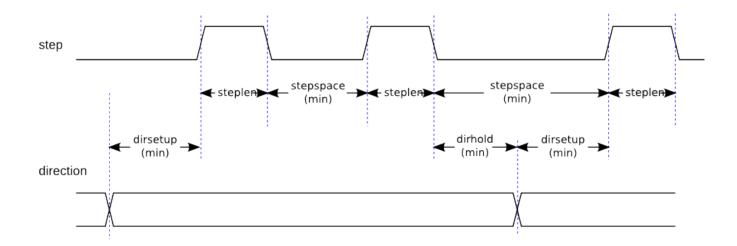
Figure 5.20 - Step and Direction Timing
