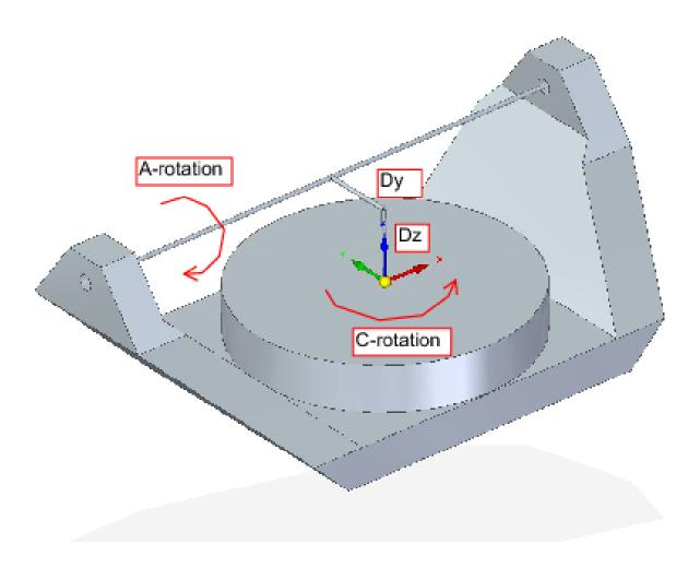
Figure 9.7 - Table tilting/rotary xyzac-trt configuration, with axis offsets
