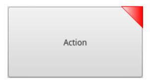
Figure 12.106 - QtVCP PushButton: Indicated Action Button, LED Indicator Option
