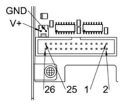
Figure 6.7 - Pin numbering of homing & end switch connector
