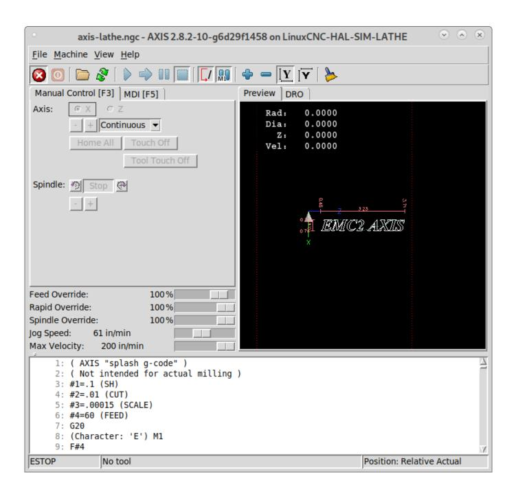
Figure 10.9 - AXIS Lathe Mode
