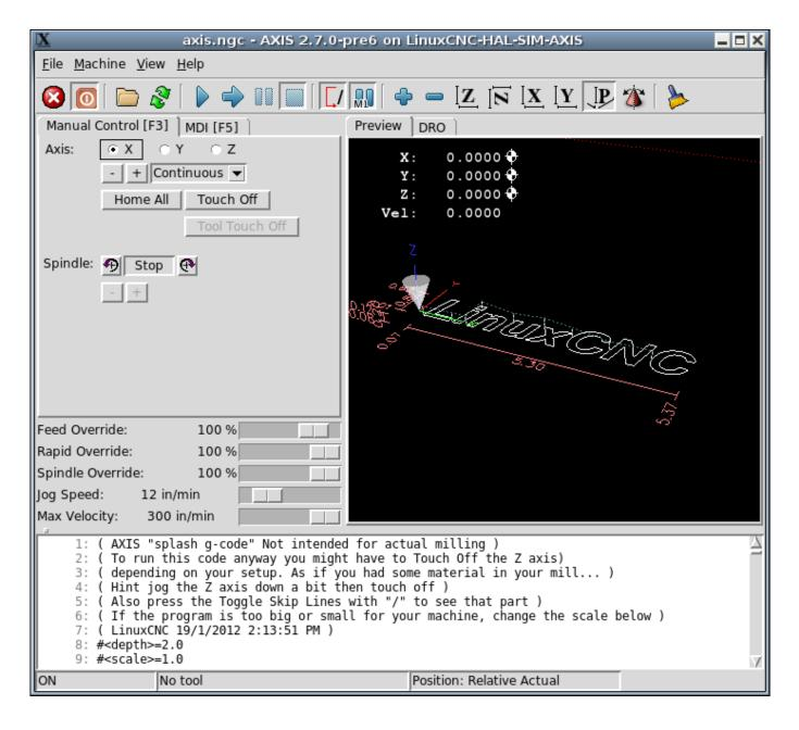
Figure 2.2 - AXIS, the standard keyboard GUI interface
