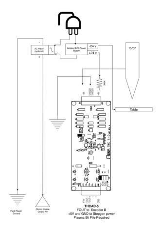
We used a 15 W Mean Well HDR-15 Ultra Slim DIN Rail Supply 24 V DIN rail based isolated power supply. This is a double insulated Isolation Class II device that will withstand any arc voltage that might be applied to the terminals.
