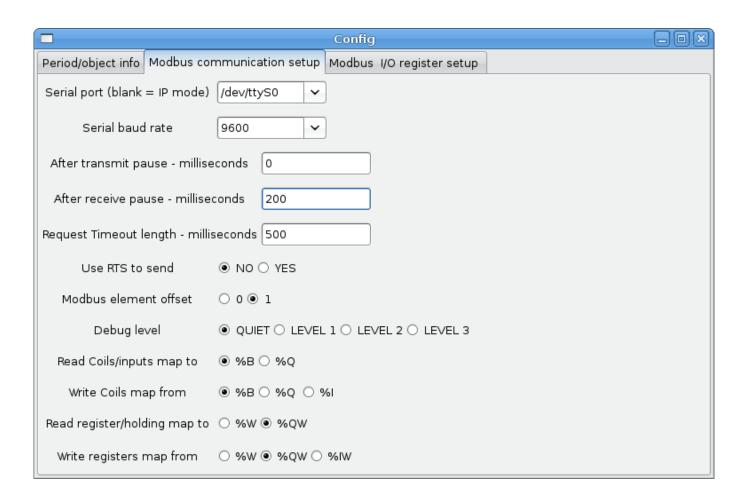
Figure 8.13 - Modbus Communication Config
