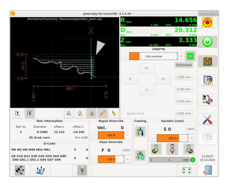
Figure 10.20 - Back Tool Lathe
