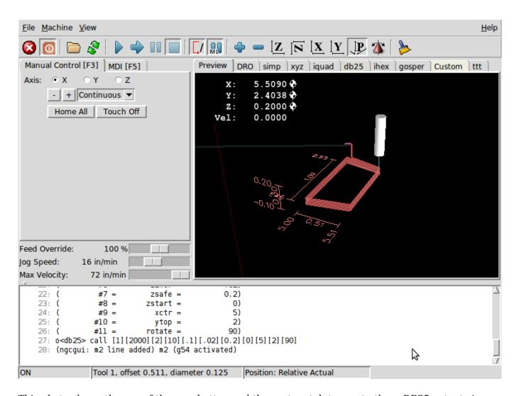
This photo shows the use of the new button and the custom tab to create three DB25 cutouts in one program.
