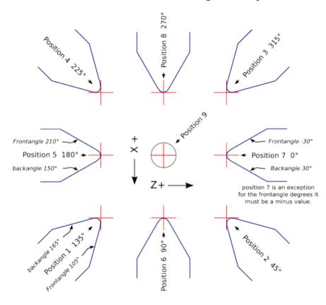
Figure 2.16 - Lathe Tool Orientations
