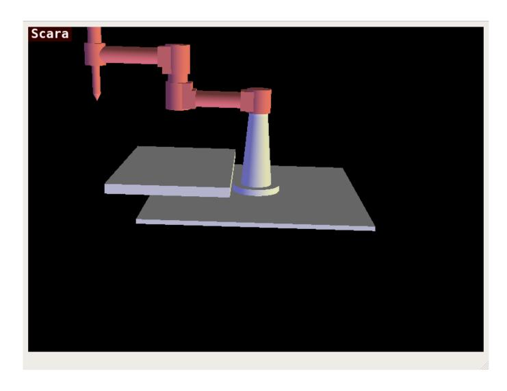
Figure 12.79 - QtVCP vismach\_scara - SCARA Mill 3D View Panel
