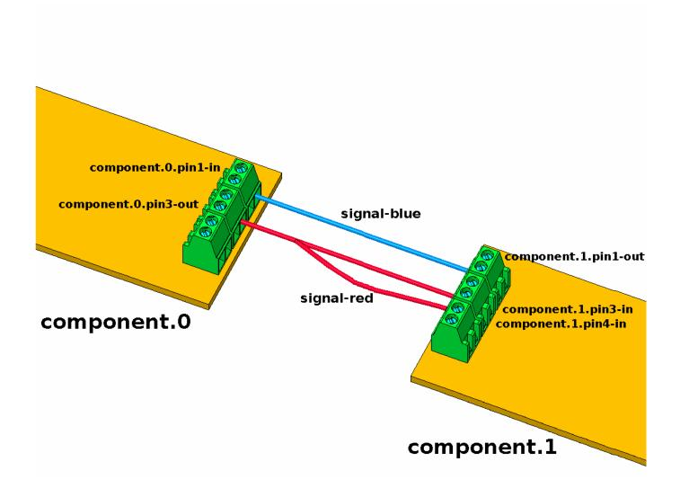
Figure 5.1 - HAL Concept - Connecting like electrical circuits.
