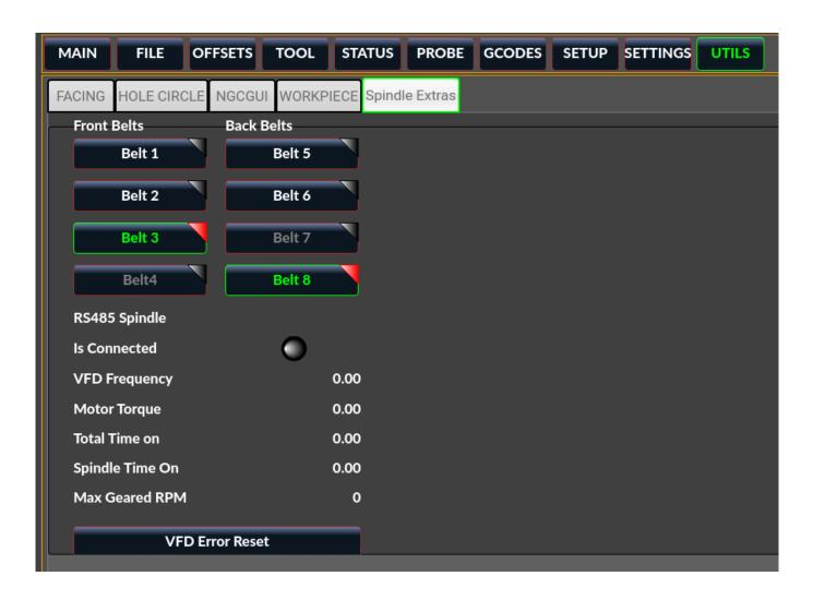
Figure 2.12 - QtVCP Example Embedded Into QtDragon GUI
