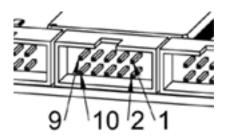
Figure 6.3 - Pin numbering of GPIO connectors
