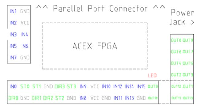
Figure 6.11 - Pluto-Step Pinout
