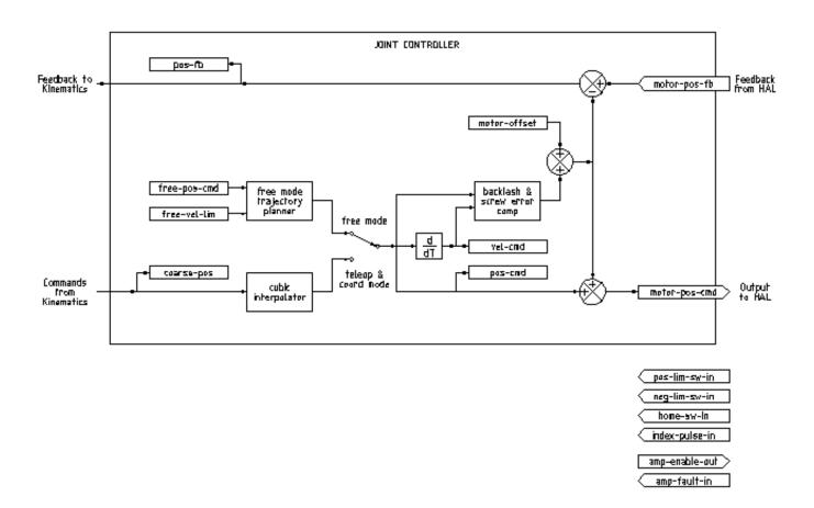
Figure 3.1 - Joint Controller Block Diagram
