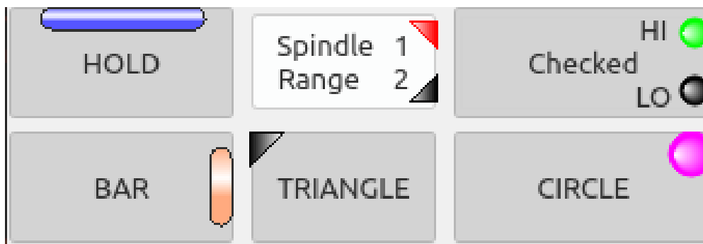
Figure 331. QtVCP PushButton : IndicatedPushButton Button, LED Indicator Option
