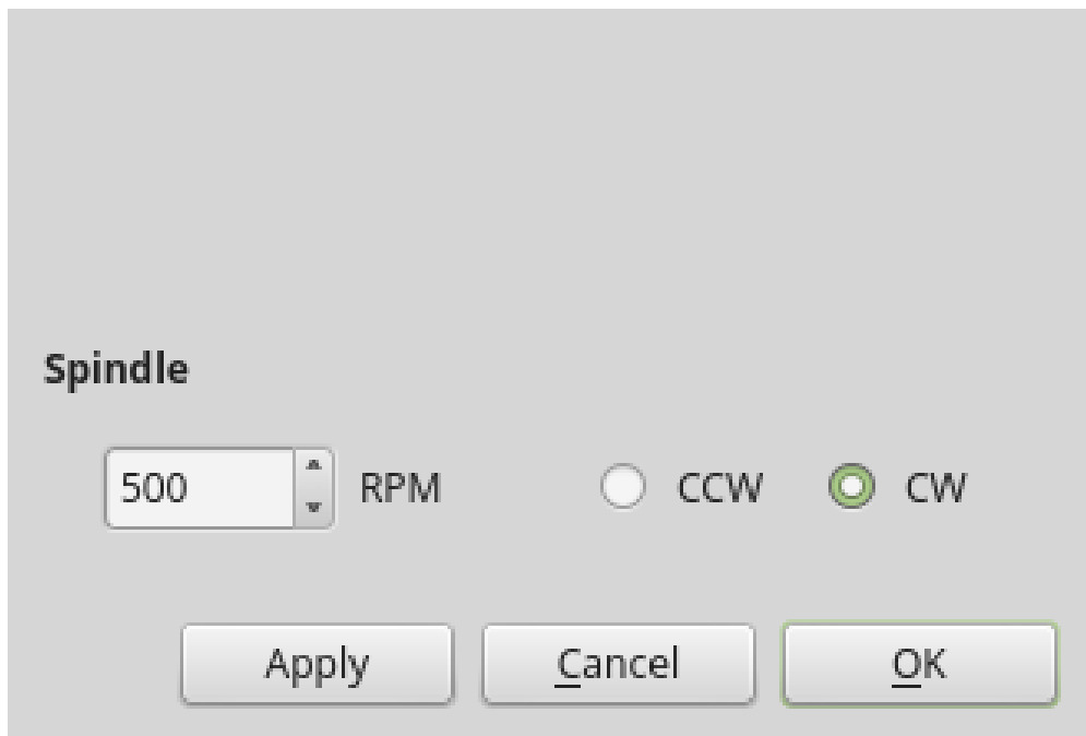
Figure 327. QtVCP RunFromLine : Run-From-Line Dialog Widget
