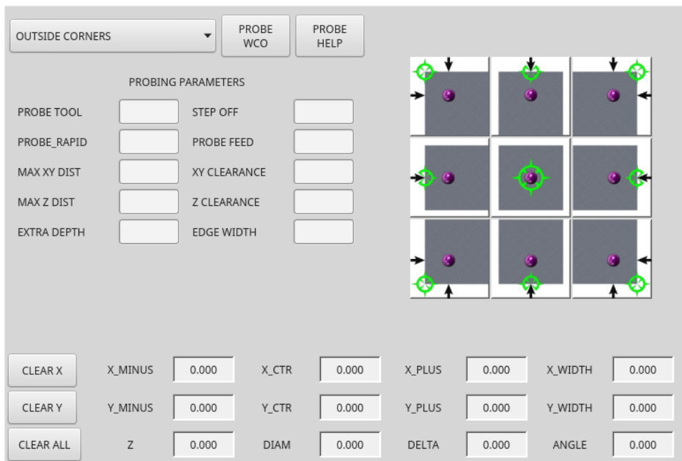
Figure 310. QtVCP BasicProbe : Simple Mill Probing Widget
